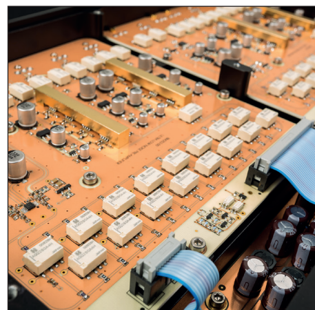
The volume control and input selection in the Bivium are carried out by relays
